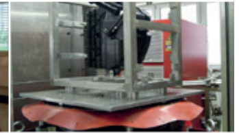
Fig. 14: Vibration test on shaker
