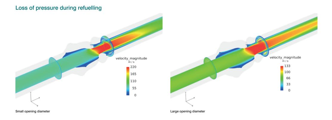
Enlargement of opening diameter by 0.5 mm
